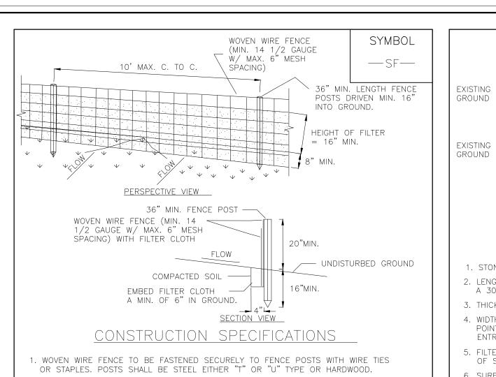
2. FILTER CLOTH TO BE TO BE FASTENED SECURELY TO WOVEN WIRE FENCE WITH TIES SPACED EVERY 24" AT TOP AND MID SECTION. FENCE SHALL BE WOVEN WIRE, 12 1/2 GAUGE, 6" MAXIMUM MESH OPENING.
